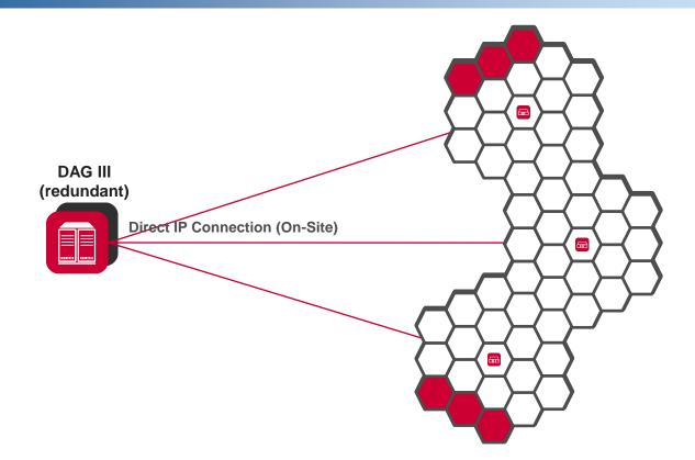
Standard Operation: Multi-Master Transmission within Net segment Wide broadcast as fallback mode if TCP/IP connection lost
