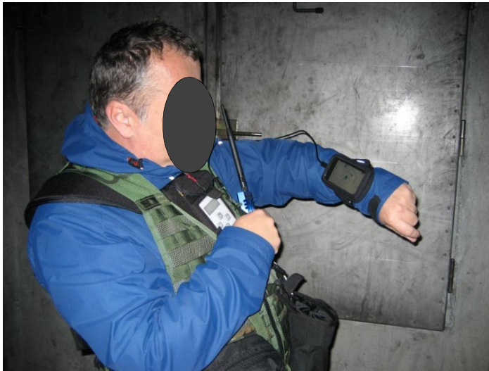
GPS positioning, inertia for indoor, sensor platform (temperature, gas etc)
