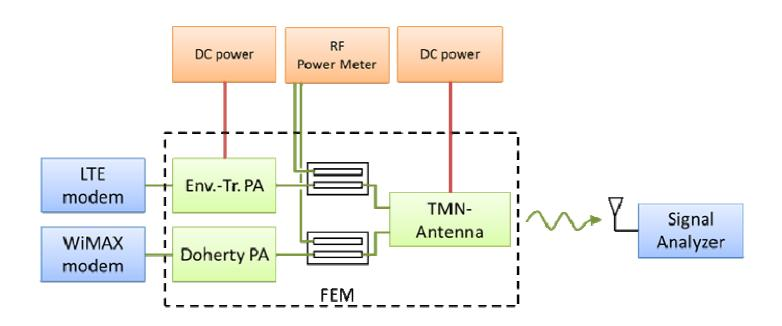
Showcase of the FEM with the Envelope-Tracking (ET) PA, the Doherty PA and the TMN-Antenna modules
